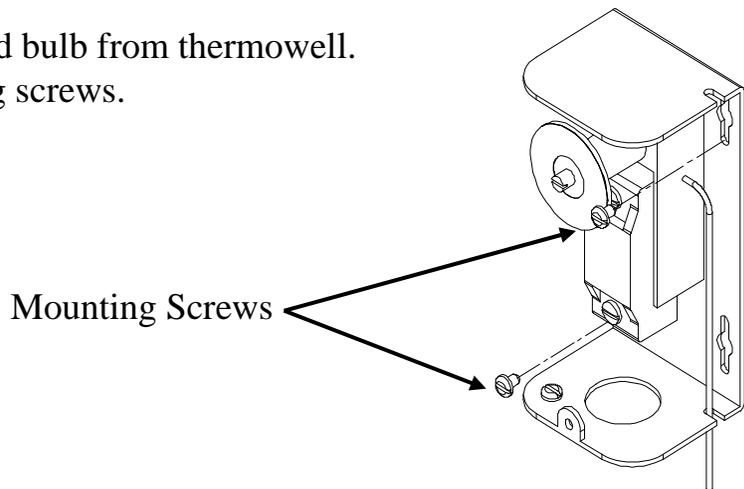
7. Replace thermostat using reverse procedure. (Note: Be sure to place capillary tube into slot in base prior to installing cover.)
