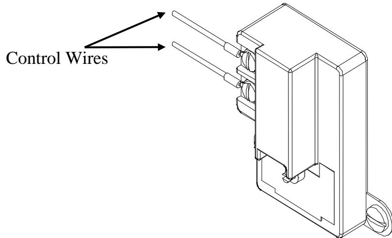
4. Remove two (2) mounting screws and disconnect from high limit cut-off, if required.
