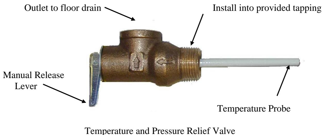
5. Install a relief valve overflow pipe to a nearby floor drain. CAUTION: No valve of any type should be installed between the relief valve and tank or in the drain line.
