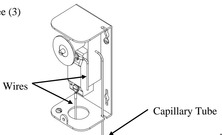
5. Remove capillary tube and bulb from thermowell.
