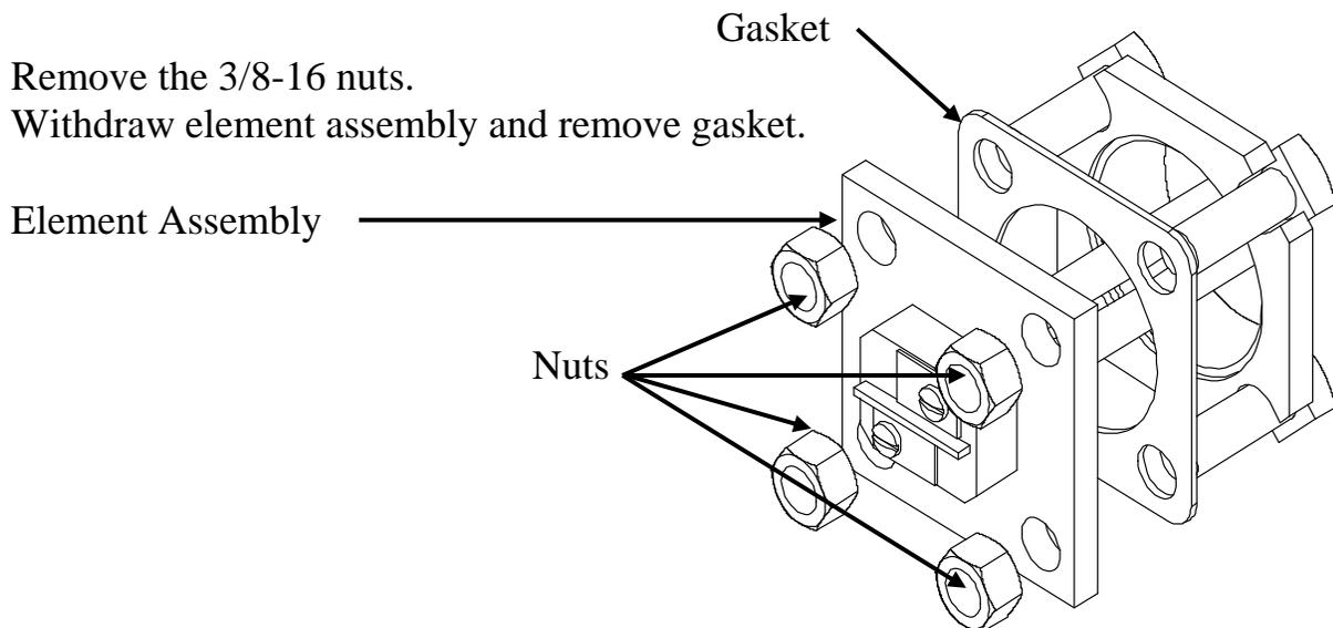
9. Install new gasket and insert new heating element.
