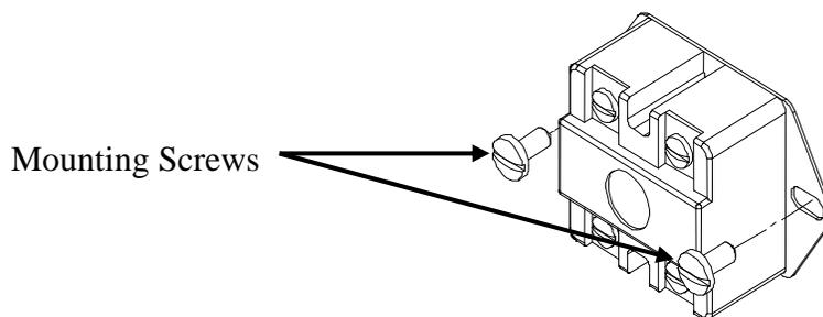
6. Replace control and install new high limit switch by performing above steps in reverse order.
