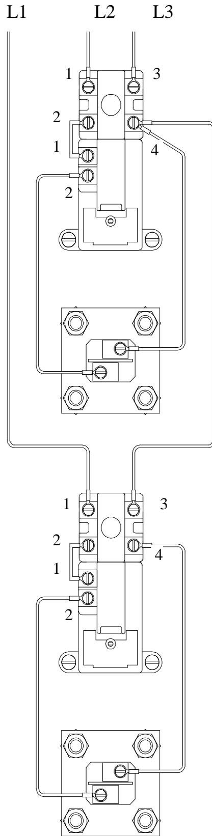
3 Ø Open Delta Wiring for Simultaneous Operation
