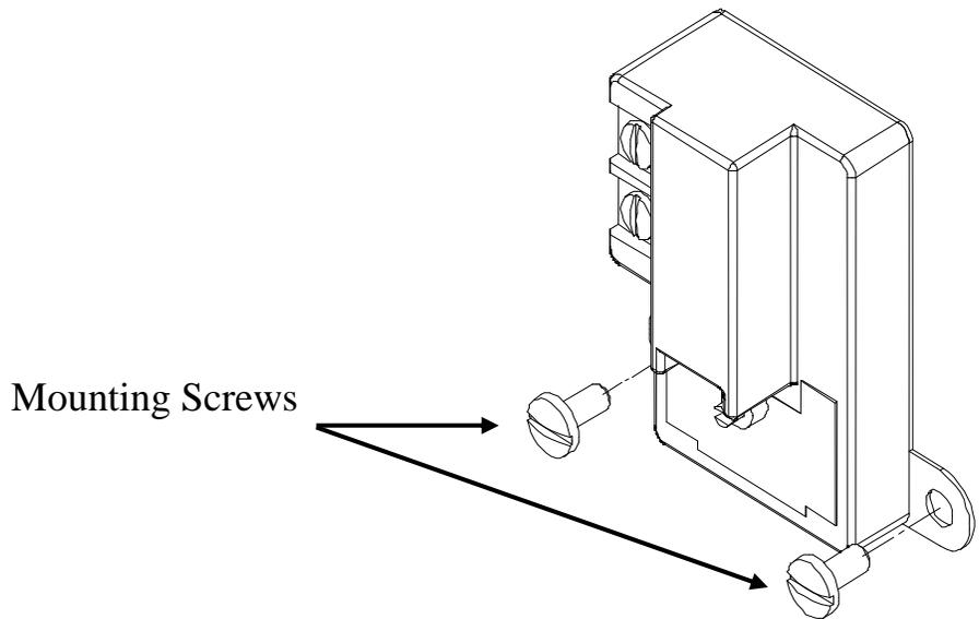
5. Replace thermostat using the reverse procedure.
